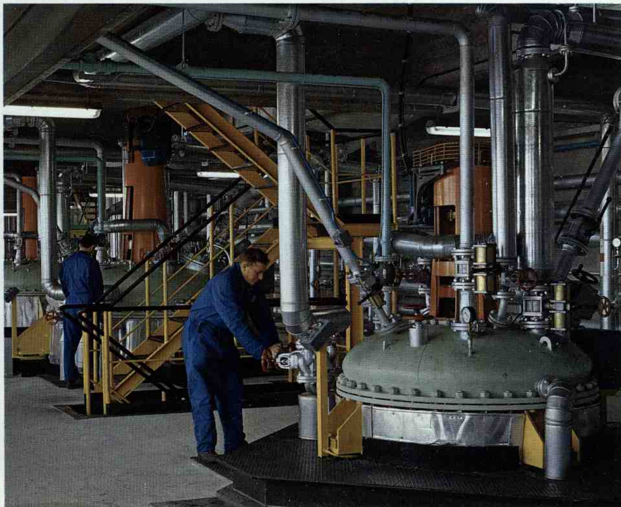
Installations for the mixing and dehydration of oils under vacuum at the new lubricants plant at Villastellone, Turin.
