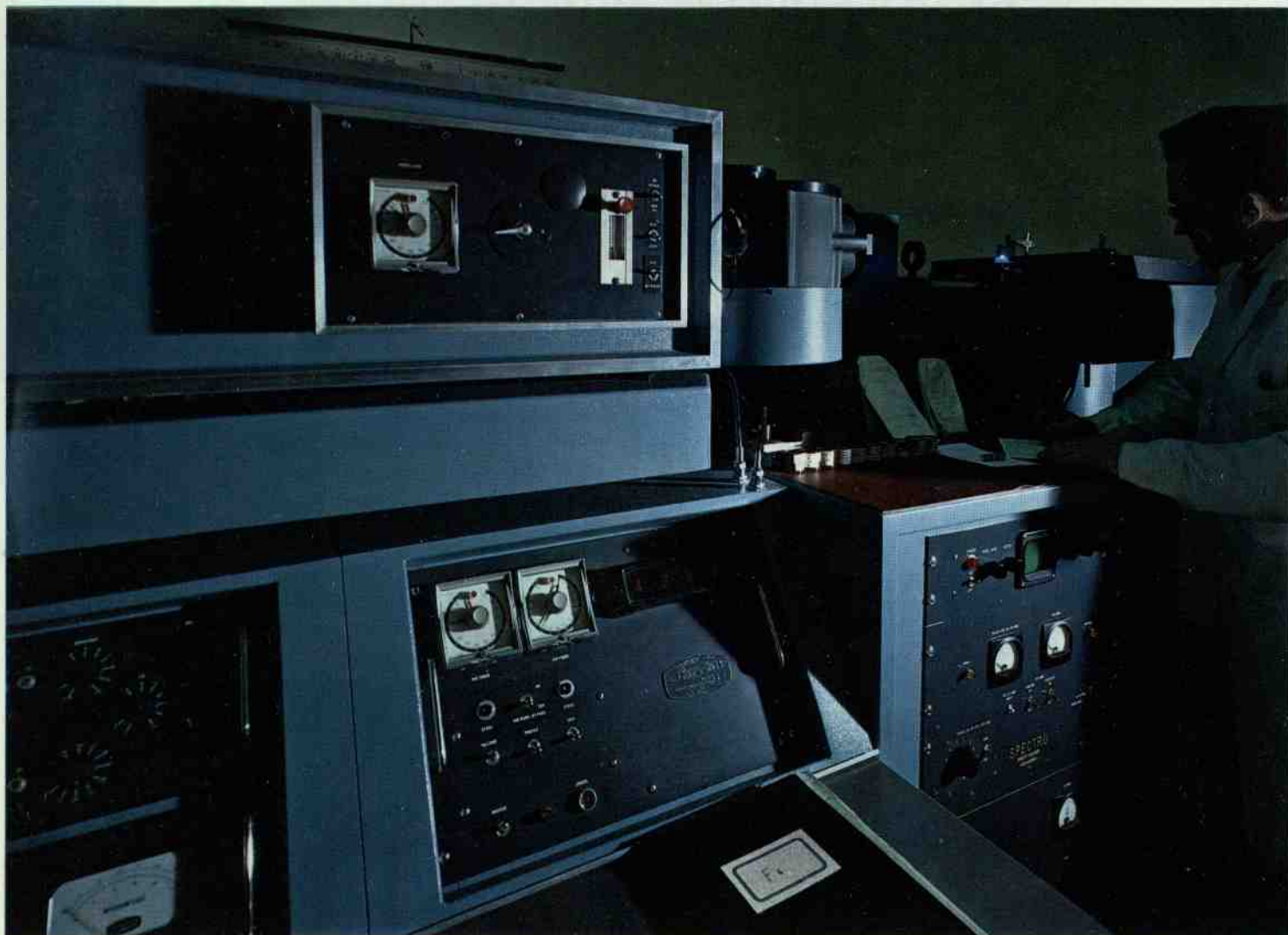
The Central Research and Control Laboratory. Direct reading spectrometer control board for the rapid analysis of metals. Complete results of analysis are available within one minute's time.
