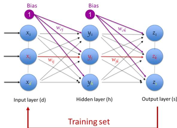
Figure 10. The backpropagation algorithm on multilayer neural network (Source: adapted from Falavigna, 2022).
